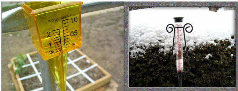
Rain gauge (amount of rain)
